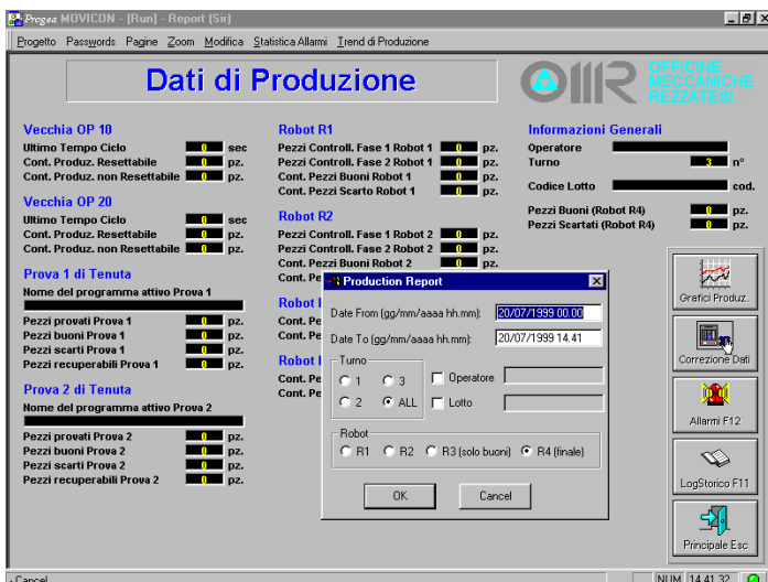
This page reports production data in realtime. The operator can use this page to get statistical production analysis by specifying the required information. Movicon creates statistical reports and production chart graphics.
