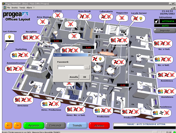
The main synoptic panel that allows the users in Progea's new headquarters to be monitored.
